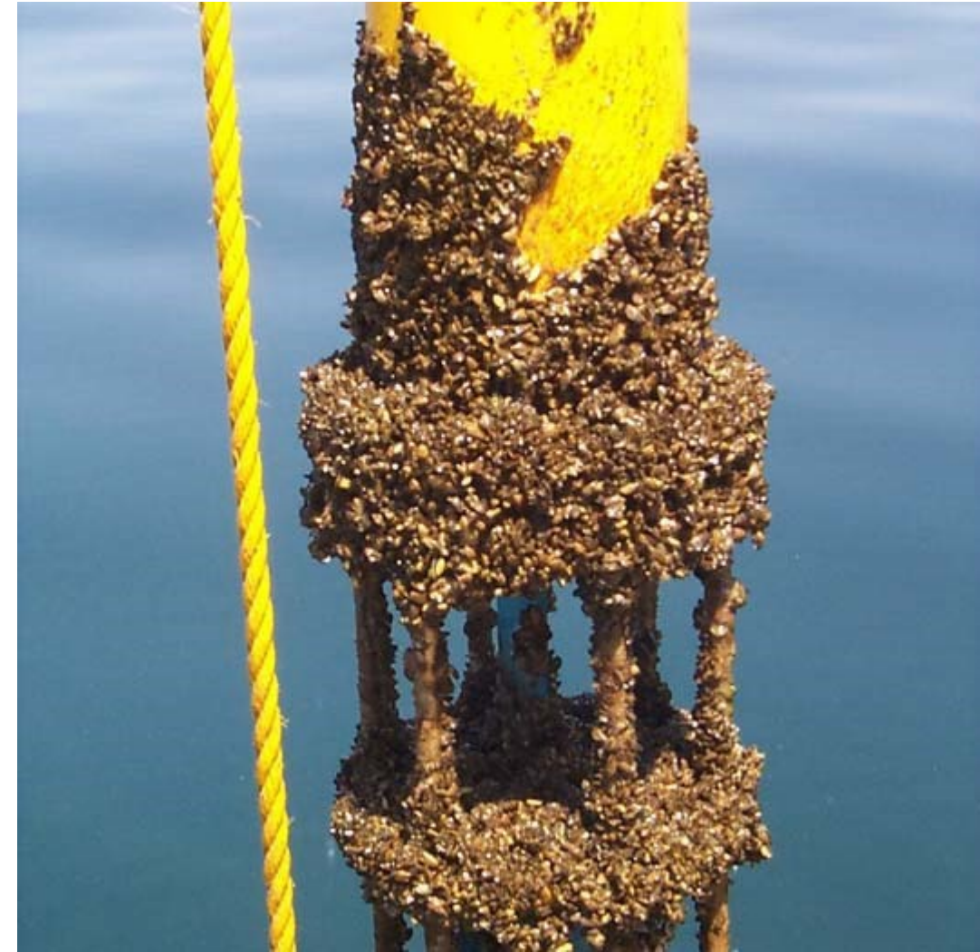
Current measurement instrument encrusted with zebra mussels
